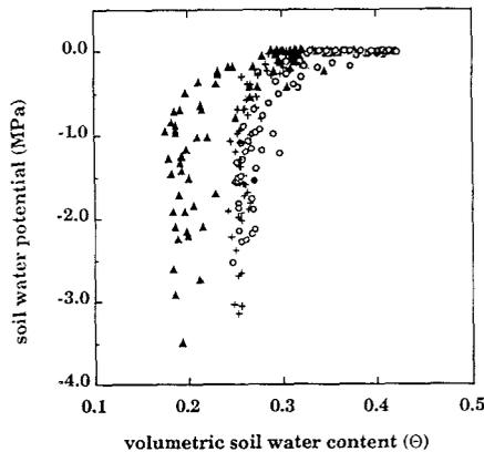
Fig. 3. Soil water retention curves established in situ by using simultaneous measurements of soil water potential (tensiometers and micro-psychrometers) and soil water content (neutron probe) at five depths (–25 cm: solid triangles, –50 to –80 cm: open circles, –110 to –140 cm: crosses). Each point represents paired observations taken using micro-psychrometre and neutron probe, on a single day. Data were obtained during 1992 and 1993 while water content fell during drought.
