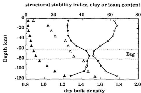
Fig. 2. Pedological description of the soil: granulometric composition in percent (clay: solid circles, loam: open circles), structural stability index (solid triangles) and bulk density profile determined using direct sampling on cylinders (open triangles).
