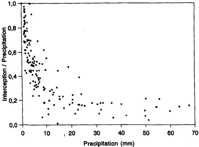
Fig. 2. Relationship between relative interception and precipitation at the event scale.
