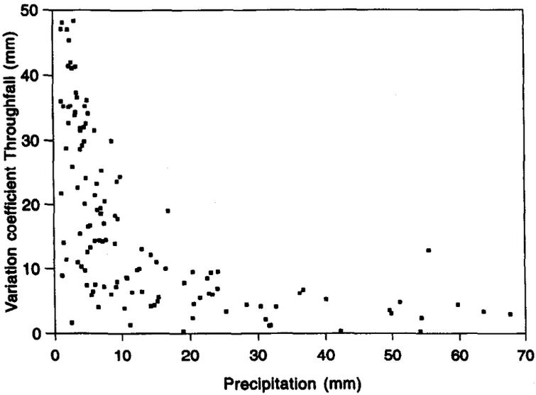
Fig. 4. Decline of spatial variation coefficient of throughfall with increasing event rainfall depth.
