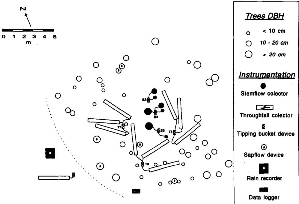
Fig. 1. General arrangement of the experimental plot for the study of forest interception fluxes at the Cal Parisa basin (Eastern Pyrenees, Spain).
